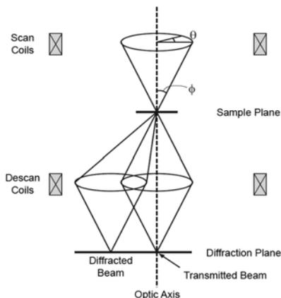
Fig 1. Precession diffraction geometry.
