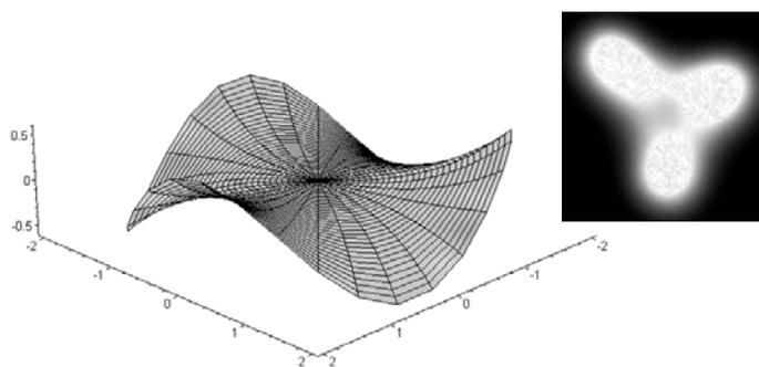
Fig. 2. Misprojection of the precessed beam by a three-fold aberration function (left) generates a star pattern in the sample plane. Image taken on JEM-2000FX.  $\phi = 40$  mrad,  $d_{lobe} \sim 25$  nm.
