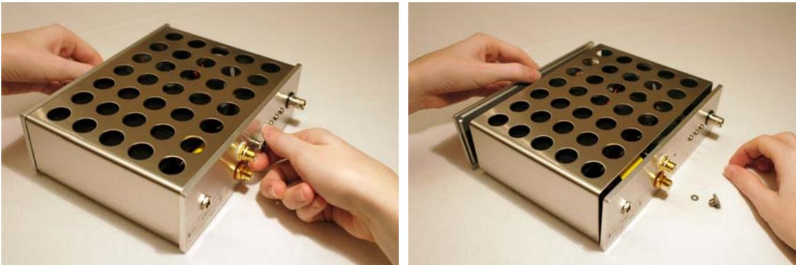
3. Pull the threaded rod through the front panel out of the dAck! 2.0. The faceplates should come loose. Like the thumb nut and washer, place the threaded rod aside.
