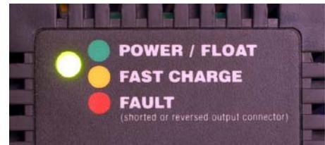
**FAST CHARGE** – When the charger is connected to depleted cells, they undergo a rapid charge cycle. At this point, the indicator should turn orange. The orange indicator will turn green when the charger enters float mode.
